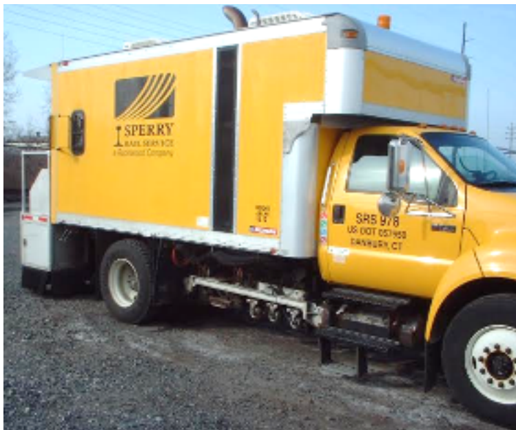
Passenger side. The rail inspection assembly can be seen between the rear tire and truck door.
