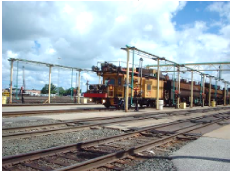
The rear of the grinding train has fire hoses to put out any fires from grinding. The two tank cars carry water to cool the rails.
