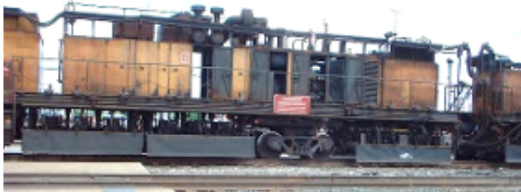
Taken in 2013 in the Collinwood yards show the rail grinding unit on the train. There were several on this train.
