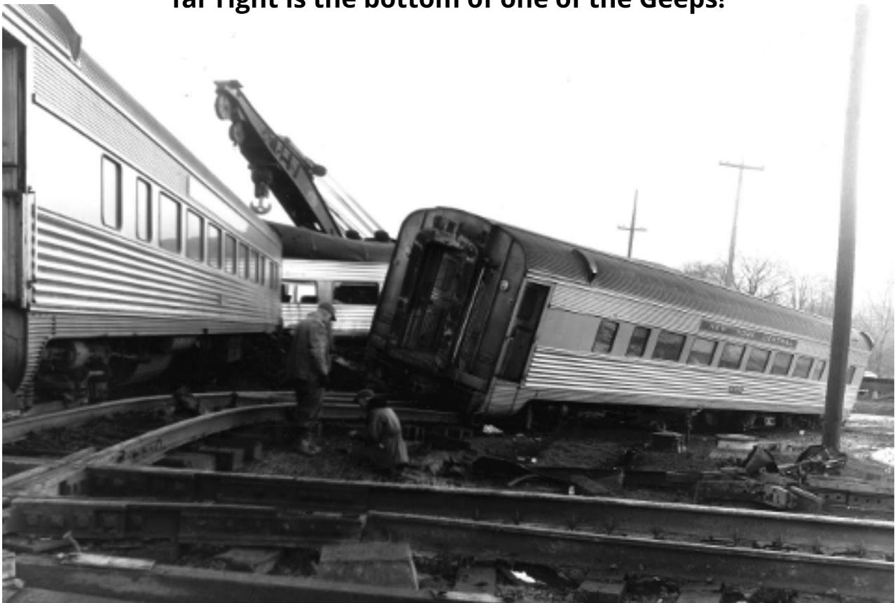
**I really would NOT like to be the two guys working next to the bent rail! Notice how the rails are lifted from the ties. The rails to the right of the crossing are also lifted, not to mention the broken rail.**
