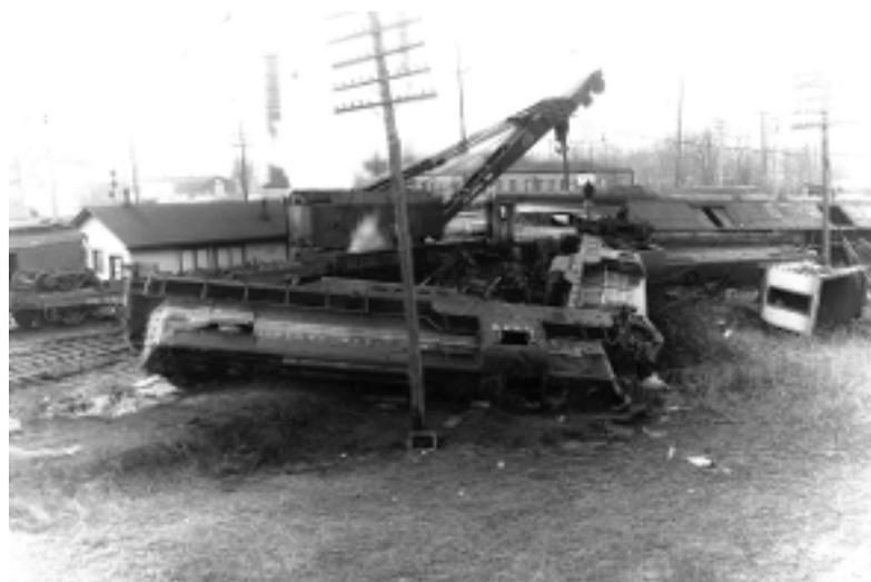
**Three GP units lie in the foreground. To the right of the engines was a unoccupied wooden tower destroyed by the wreck. Notice that the hook was brought in from Collinwood Yards.**
