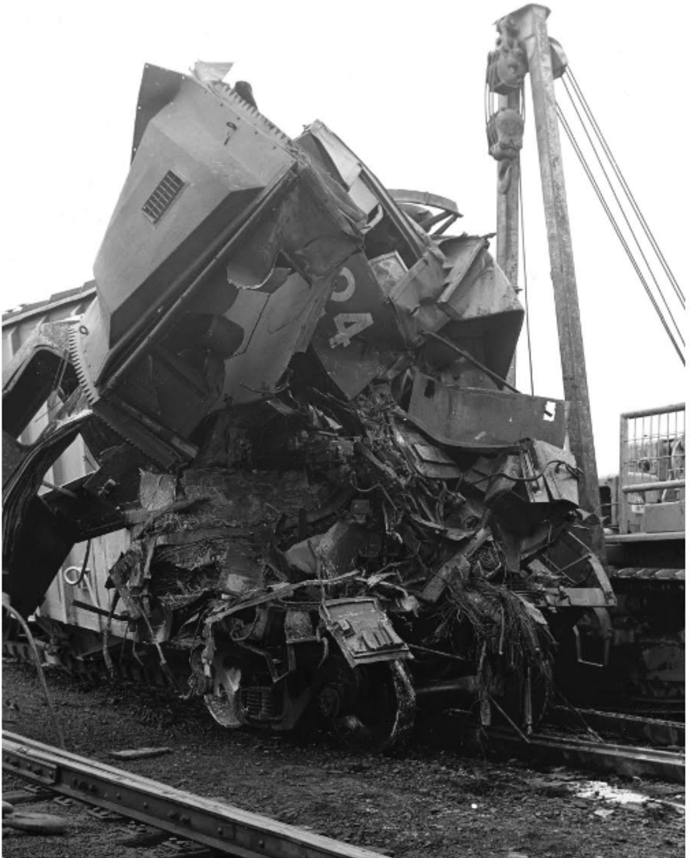
The force from impact hitting the bridge is seen in this image of the second unit.
